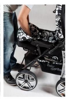
Lift the handle upwards until you hear the typical "click" sound of the locking devices.
